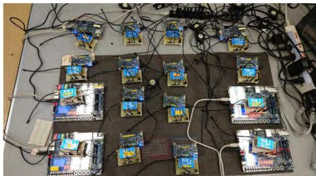
Fig. 8 Experiment of shared memory and distributed processing on FPGA multihops
