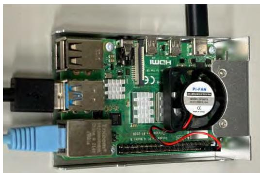
Fig. 5 Photograph of Raspberry Pi 4B.
