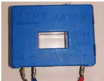
Fig. 3 Photograph of current transducer LA55-P.
