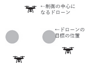
Fig. 3(3) Control by relative positions
