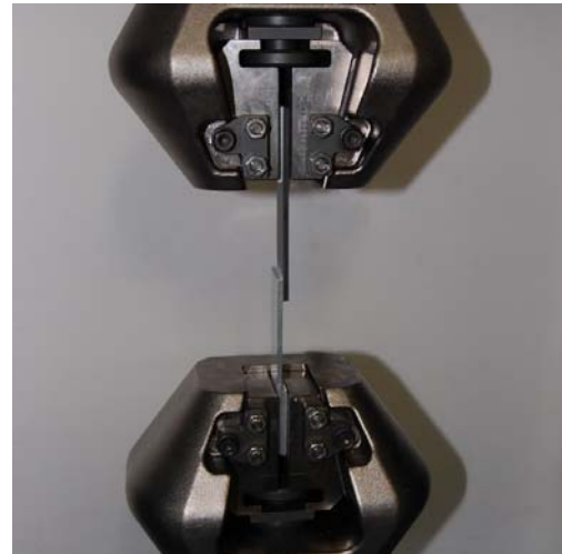
Fig.4 Experimental setup of tensile shear test
