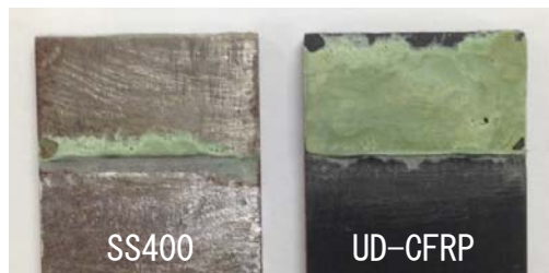
Fig.12 Fracture surface in the case of UD-CFRP/SS400 joint
