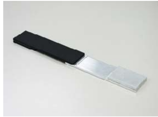
Fig.2 Fabricated joint specimen, "UD-CFRP/A6063 joint"
