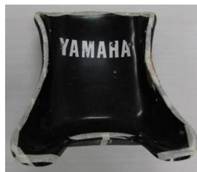
Fig.4 GFRP go-cart seat(weight 1510g)
