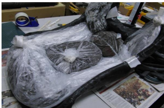
Fig.16 CFRP sandwich sheet forming (sand bag weight)
