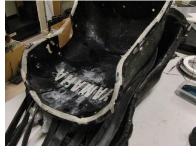
Fig.18 GFRP sheet as forming punch
