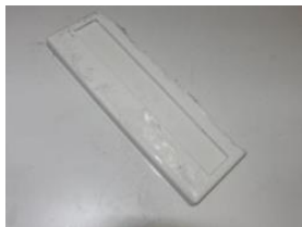
Fig.7 Silicone rubber mold for CFRP test piece
