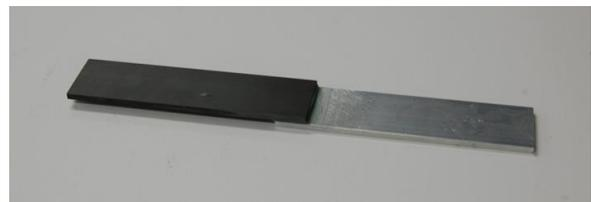
Fig.4 Joint specimen fabricated by UD-CFRP and A6063
