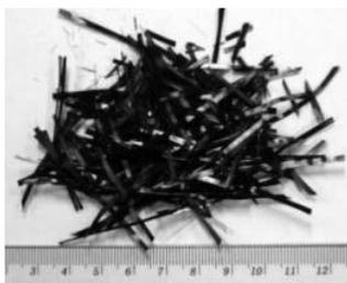
Fig.1 Cutted carbon fibser bunch (3K)
