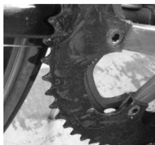
Fig.24 CFRP chain sprocket (after 650km running test)
