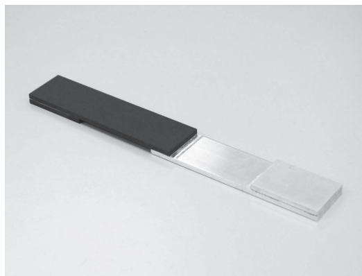
Fig.4 Single-lap joint bonded by structural adhesive.
