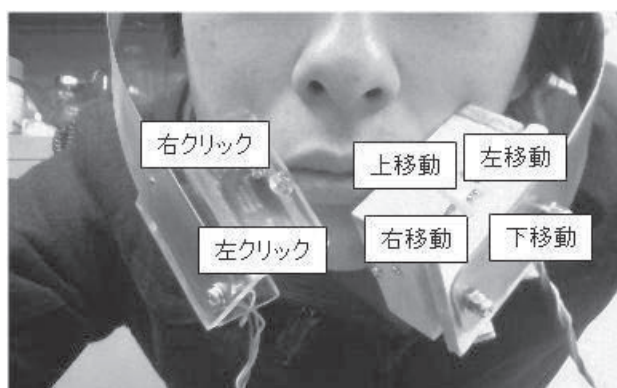
Fig.11 The improved interface which is able to operate the pointer on the desktop to diagonal directions
