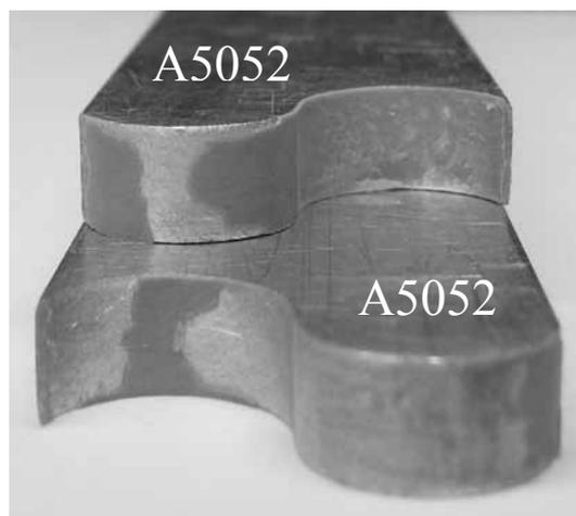
Fig.10 Fractured surface of joint specimen in case of similar adherend (A5052 - A5052).
